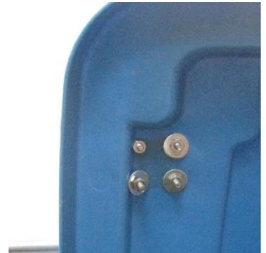
1. Pre-drill  $\frac{3}{8}$ " holes for the hasp hinge in the two top, front corners (A) of the body of can.
