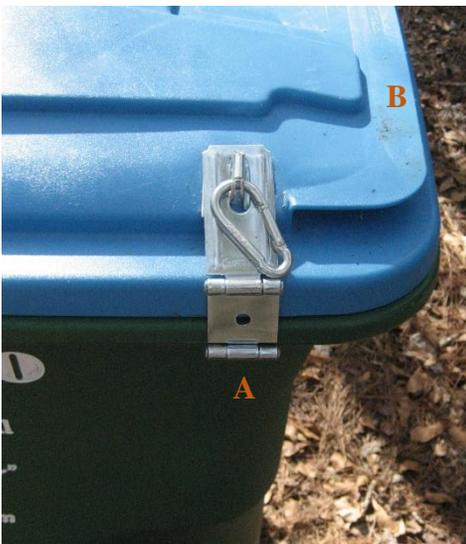
3. Lay the hinge over the lid to mark the best position for the eye of the hasp. Make sure the hinge can be locked and unlocked easily. Pre-drill  $\frac{3}{8}$ " holes in the marked spots on the lid of the can for the hasp eye.
