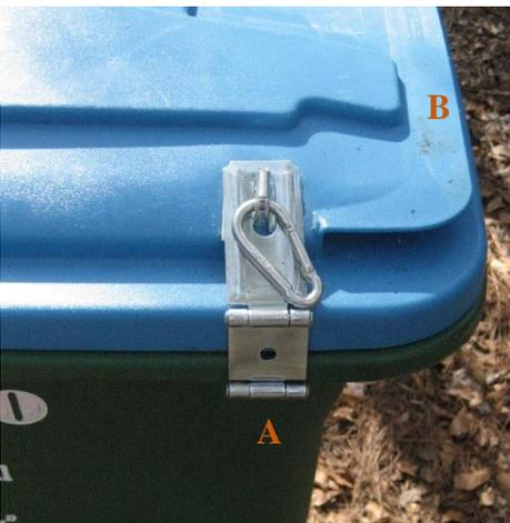
3. Lay the hinge over the lid to mark the best position for the eye of the hasp. Make sure the hinge can be locked and unlocked easily. Pre-drill 3/8" holes in the marked spots on the lid of the can for the hasp eye.
